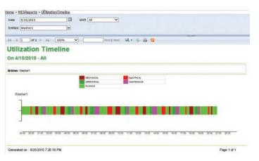
Automatic utilisation event and reason capturing allows users to record short stoppages and frees up operators from manual data entry. Pareto graphs display rate counts, durations of utilisation states and reasons associated to line or equipment performance.
